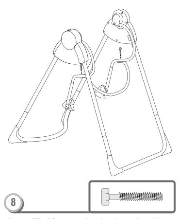
• Insert an M5 x 2,9 cm screw through each seat tube and the seat tube support.
